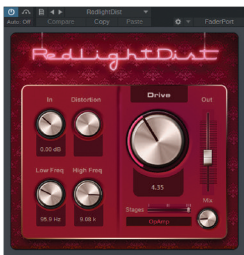
Figure 3: The RedLightDist distortion plugin bundled with PreSonus Studio One. Note the Mix wet/dry control in the bottom right.
